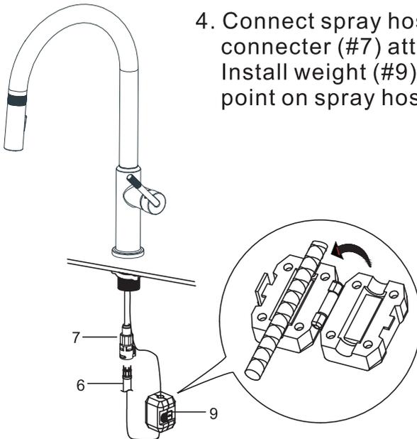
4. Connect spray hose (#6) to quick connector (#7) attached to supply line. Install weight (#9) on lowest vertical point on spray hose (#6).
