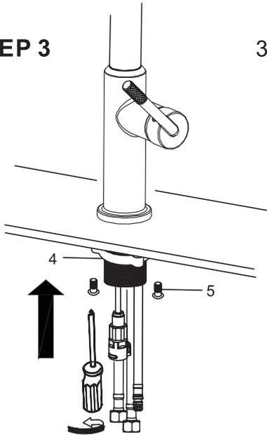
3. After adjusting the direction of the main body, tighten the mounting nut (#4) with hands and tighten the mounting screws (#5) with a Philips screwdriver.
