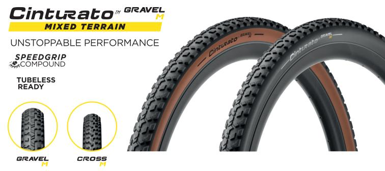
Medium profile and tread spacing for riding quickly and confidently over a **mixed** variety of **terrains**, from hard to soft, whether for **dry** or **wet**.
