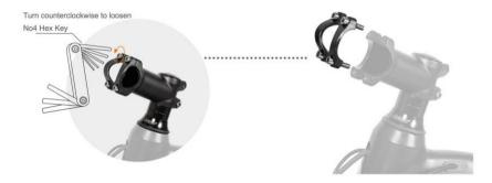
2. Set up the handlebar. Place in handlebar, then set up the front attachment as shown. Make sure the brakes are at an  $45^{\circ}$  to the ground.
