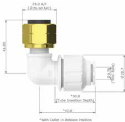
800-02214 JG WATERMARK BENT TAP CONNECTOR 12MM PEMBTC1214 1/2 BSP
