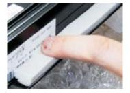
2. Apply foam tape all the way around the mainframe flange. Top corner of the window is a suitable starting point. Take particular care around the 2 radius corner. Cut off tape end at the starting point to form a continuous seal. Join foam tape, cleanly, as above. Apply bead of silicone to foam tape.
