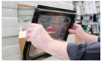
3. Fill cladding seams with silicone then crush final 10mm. Position window in opening of the van where it is going to be permanently installed. Do this from the outside of the van. Bottom of the window to go in first - to clear thumb locks.
