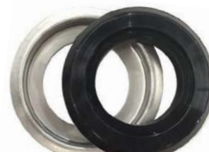
494015 Grease Seal Marine 2/2.5/3T Suits nominal housing diameter: 89.96mm Seal Journal: 60.3mm
