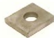
590510G Spring pad to suit round and square, Galvanised L 47mm W 40mm T 8mm
