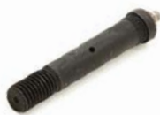
590711 Centre rocker pin M18 x 100mm greasable suit tandem 60mm rocker springs D 18mm L 100mm
