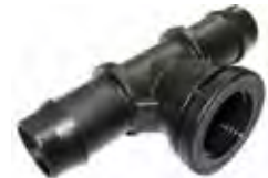
800-02348 19MM BARBED X 1/2" BSP FEMALE THREADED TEE
