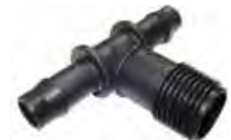
800-02352 13MM BARBED X 1/2" BSP MALE THREADED TEE
