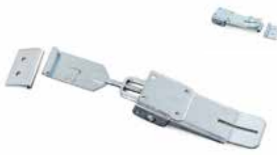
Camper Roof Clamp Lockable This clamp is commonly used on pop top caravans and wind up campers to hold down the roof while the trailer is in storage or while travelling. FEATURES: • Includes toggle clamp, space for lock and extra locking bracket suitable for a small padlock (not included) • Zinc plated Colour Silver 008267
