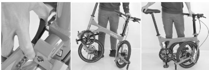
Step 3. Open the seat post quick-release, slide the post to the bottom and closed the quick-release.
