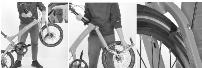
**Step 2.** Release the rear swing arm catch, lift the saddle to let the rear swing arm rolling forward, turn the handlebar to let the front wheel rest against the rear wheel.
