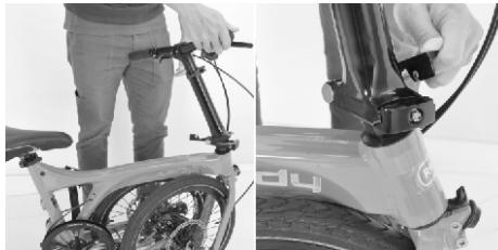
Step 2. Open the seat post quick-release, pull the seat post to the appropriate height (please see the height indicator on the post), be careful not to exceed the safety line, close the quick-release, and rotate the handlebar to make the front wheel in 90 degrees.
