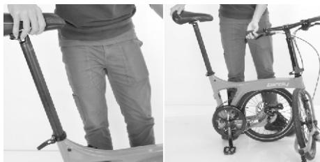
Step 3. Lift up the saddle, swing the rear fork backward and ensure the rear swing arm catch is engaged.
