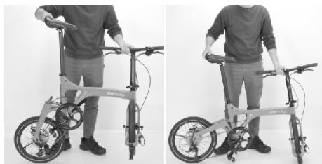
Step 4. Lift up the stem, unfold the front fork, and engage the spring onto the front swing arm catch.
