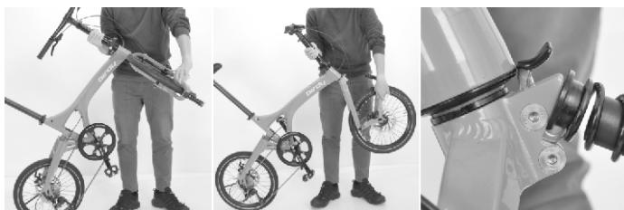
**Step 5.** Check if the brake cable and gear cable twine together, and if the chain drops.
