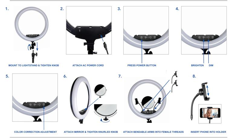
1) Mount light to any light stand with a 5/8" spigot and tighten using the knurled knob on the side of the light stand adapter.
