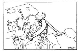
(e) Install two new gaskets, the EGR valve adaptor and air pipe (LN only) with the four nuts.
