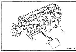
(b) Lift the cylinder head from the dowels on the cylinder block and place the head on wooden blocks on a bench.
