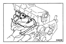
(b) Remove the four bolts, four nuts, exhaust manifold and gasket.
