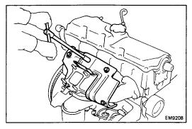
(c) Install the two heat insulators with the four bolts and nut.
