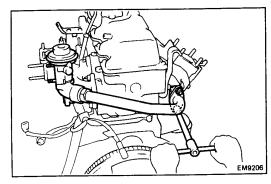
(d) Remove the two nuts, EGR valve with the pipe and gasket.
