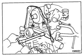
REMOVE NO. 2 TIMING BELT COVER Remove the four bolts and belt cover.
