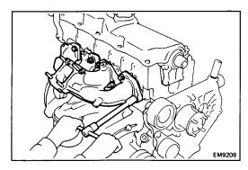
(b) Install the exhaust manifold with the four nuts and four bolts.
