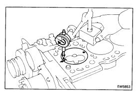
(e) Measure the piston protrusion from the cylinder block by sliding the dial indicator.
