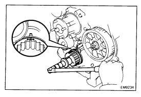
(c) Find where the piston head protrudes most by slowly turning the crankshaft clockwise and counterclockwise.
