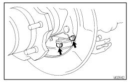
(f) Remove the 2 bolts and parking brake bellcrank assembly.
