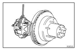
(b) Suspend the disc brake assembly securely. Ensure that the hose is not stretched.
