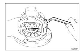
(e) Install the pinion shaft pin and washer.
