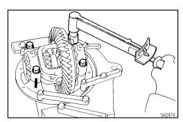
(i) Torque the 4 bearing cap bolts.
