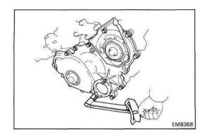
(c) Install the timing gear cover with the fourteen bolts.
