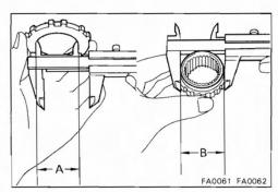
3. MEASURE OIL CLEARANCE BETWEEN INNER HUB AND FREE WHEELING HUB RING
