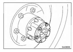
(d) Install and torque the cover mounting bolts.Torque: 100 kg-cm (7 ft-lb, 10 N·m)
