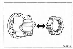
2. INSPECT BODY AND CLUTCH Check that the clutch moves smoothly in the body.
