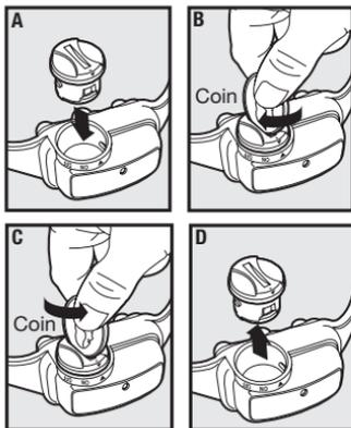
This Bark Control Collar utilizes a replaceable PetSafe® battery (RFA-188). This unique battery is designed to make battery replacement easier and increase water protection.
