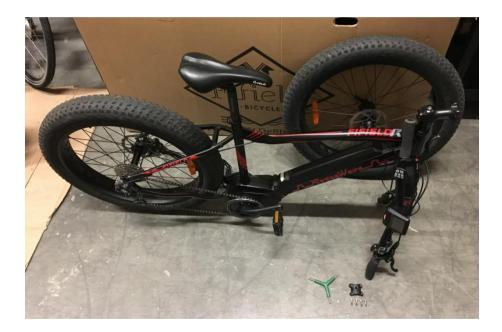
2. Next, use the depicted tool below to attach the handle bars using the handle bar bracket. This is done by holding the handle bars in place, and then using the 4 screws to hold it in place (see following image).
