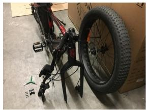
5. Once the fork is resting on the skewer, tighten as needed. Make sure it is firm, but loose enough to fold the right side lever inwards.
