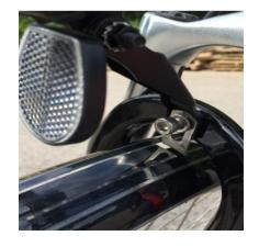
Note: When looking at the metal extension the fender has a short end and a long end. The long end goes to the back of the wheel to protect your legs from water, dirt, etc.
