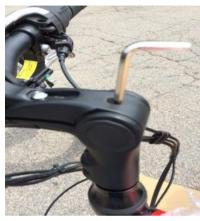
4. The handlebars are currently positioned at a 90 degree angle; bring the handlebars to a straight position perpendicular to the ground. Locate the two4mm bolts on the side of the handlebars. These bolts are used to lock the handlebars in place. Make sure that the handlebars are in an appropriate riding position with the fork and use the allen wrench to tighten.
