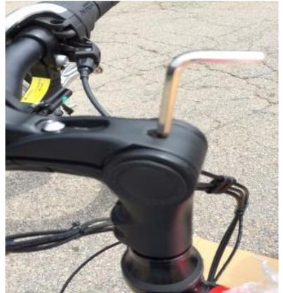
4. The handlebars are currently positioned at a 90 degree angle; bring the handlebars to a straight position perpendicular to the ground. Locate the two 4mm bolts on the side of the handlebars. These bolts are used to lock the handlebars in place. Make sure that the handlebars are in an appropriate riding position with the fork and use the allen wrench to tighten.
