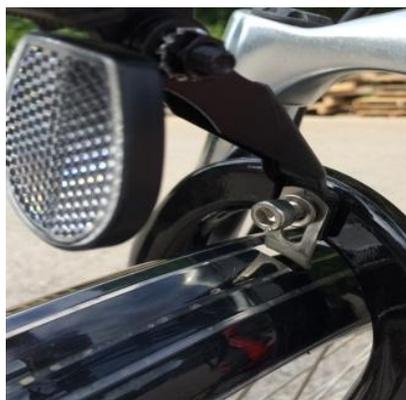
**Note: When looking at the metal extension the fender has a short end and a long end. The long end goes to the back of the wheel to protect your legs from water, dirt, etc.**
