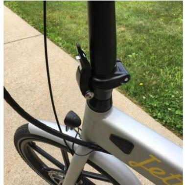
Next, use the depicted tool below to loosen the 2 screws on the handlebar clamp just enough for you to roll the handlebars toward the seat until they are in the correct position (shifters facing you at the right level and the LCD facing up toward your face). Make sure to then tighten down the screws.
