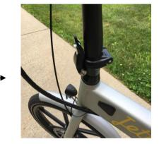
Next, use the depicted tool below to loosen the 2 screws on the handlebar clamp just enough for you to roll the handlebars toward the seat until they are in the correct position (shifters facing you at the fight level and the LCD facing up toward your face). Make sure to then tighten down the screws.
