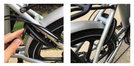
In the above image on the right the lock is in the closed position, seen by the silver bolt that loops through the rims and into the other side.
