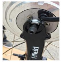
7. Place the washer over the bolt, followed by the lock washer, and finally tighten the nut to secure the wheel properly. Use a 15mm wrench to tighten. When both nuts are fully tightened, return the bike to its original upright position and put the kickstand down for the remainder of assembly.
