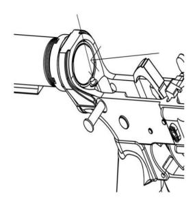
b. Depress the buffer retainer pin to permit the buffer and the spring to move forward. Depress the hammer to allow the spring and the buffer assembly to continue moving forward and be removed from the receiver extension.
