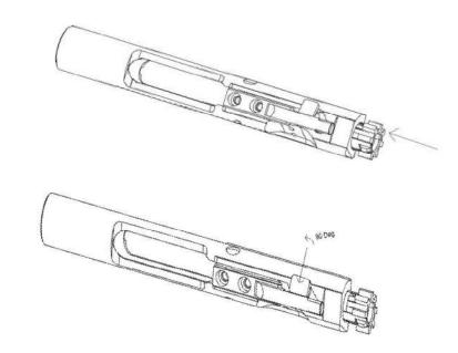
a. Remove the cam pin by lifting it out away from the bolt carrier.
