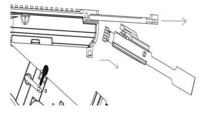
a. Remove the charging handle by pulling it backwards to keyway and then down and out of the upper receiver.
