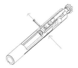
a. Tilt the bolt face up and remove the firing pin.
