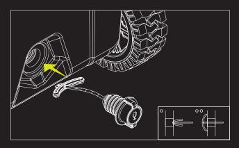
Loosen and pull out the drain plug until the stopper is engaged. Tilt the cooler at an angle to ensure you drain the cooler completely.
