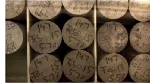
Comprehensive testing in our in-house laboratory enables us to meet or even exceed ASTM/CSA required standards. This include freeze-thaw testing (stress/weather resistant tests) and solar reflectance index, among other tests. These data points and corresponding results also allow us to react and respond to any customer inquiry concerning our products.
