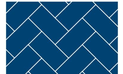
**Interesting Fact:** Historically, testing has shown that herringbone patterns (as detailed in the figure above) are best for maintaining interlock – with the 45° pattern being the most effective in heavy vehicular applications.
