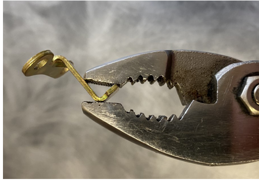
Photo 10 - Bend wire retaining clip to add more tension to wire
