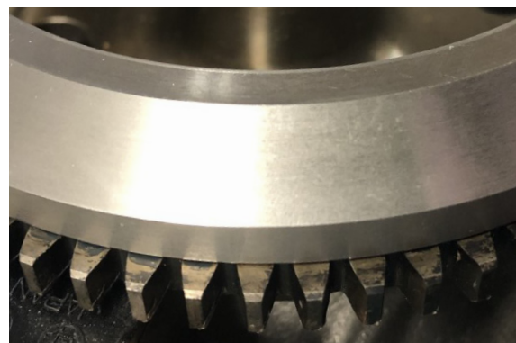
Photo 10 - Snug down and begin to tighten press tool. Tighten 1/2 turn. Tap press plate to help align the gap. Weight ring stops moving when pressed all the way on.
