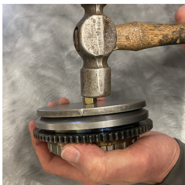
Photo 9 - Tap press plate every 1/2 turn to help aid alignment.
