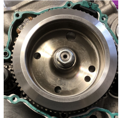
Photo 2 - Weight ring mounted to rotor.
