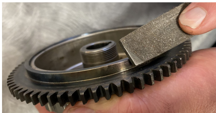
Photo 5 - File sharp corner on rotor.
