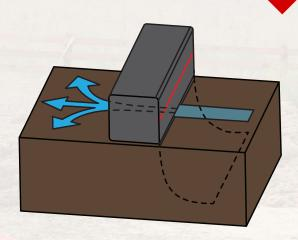
The outer layer of monofilament fabric filters the sediment laden water as it passes through the base of the wattle above the "tail section". The estimated clean water flow-through rate is 100gpm/ft². DuraWattle is designed to dewater and retain sediment while dissipating concentrated flow into more manageable sheet flow.
