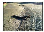
Fiber Rolls were installed first on the site and failed in the first storm
