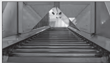
24" wide conveyor chain with 3/8" bars
