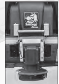
High flow chute with larger 14 in. spinner, open trough, and adjustable height and spinner shield
