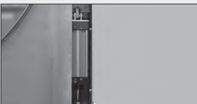
Dual air tailgate cylinders standard
