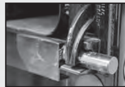
3008560 - Optional Dump Tail Gate Latch Kit
