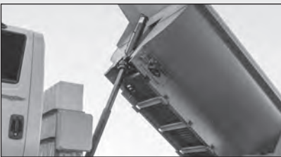
Mailhot® multi-stage, double-acting, nitrided cylinder, trunnion-mounted hoist
