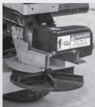
STANDARD LENGTH CHUTE Features high flow chute with larger 14" spinner, open trough, and NEW stainless steel spinner shield
