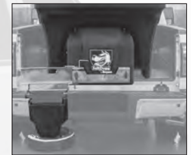
Swing-away chute for bulk unloading
