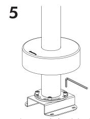
Now you have to screw firmly on the base flange Visser maintenant fermement à la base de plancher
