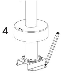
Place the base flange, mark the position of the anchors or screws
