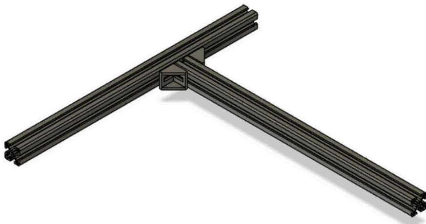
5. Insert T-nut and slide rod clamp into the rail. Adjust position at halfway (12" from the end of the rail), or as desired. Tighten rod clamp
