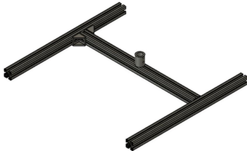
7. Adjust positioning as desired and make sure the placement is even. Tighten the corner clamps once the base is square.
