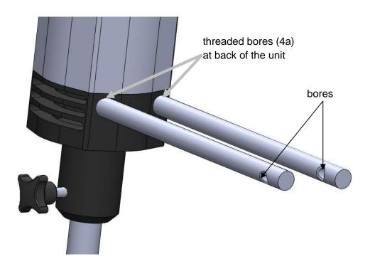
Screw the support rods (4) into the threaded bores (4a) at the back of the unit.
