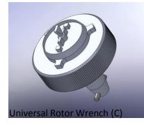
For undoing the rotor (1), use the two special wrentches (to be ordered separately). The socket wrench (B) is used to counter-hold the Shaft, and the rotor wrench (C) to undo the rotor (1). To exchange the stator (2), remember that the fastening thread is **counter-clockwise**.
