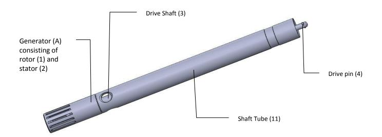
The shaft cannot be used alone. Only combinations of shaft and generator (A) can be used for working with a medium.
