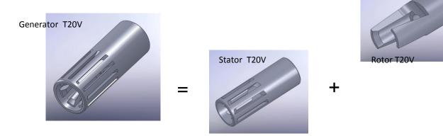
To create a **V-type generator** use a V-rotor plus a V-stator. This combination is suitable for coarse media.
