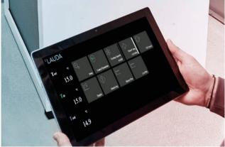
An integral web server gives the user the option of viewing or modifying settings by calling up the IP address in any standard web browser.
