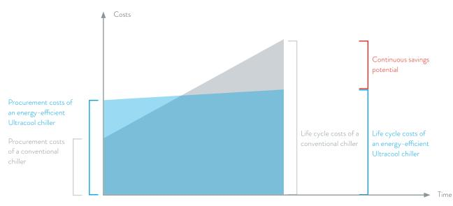
Long-term savings potential with the latest generation of energy-efficient Ultracool circulation chillers
