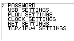
3. Use the **Down** button to select "TCP/Ipv4 SETTINGS" and press **Enter** to access the IP Configuration screen:
