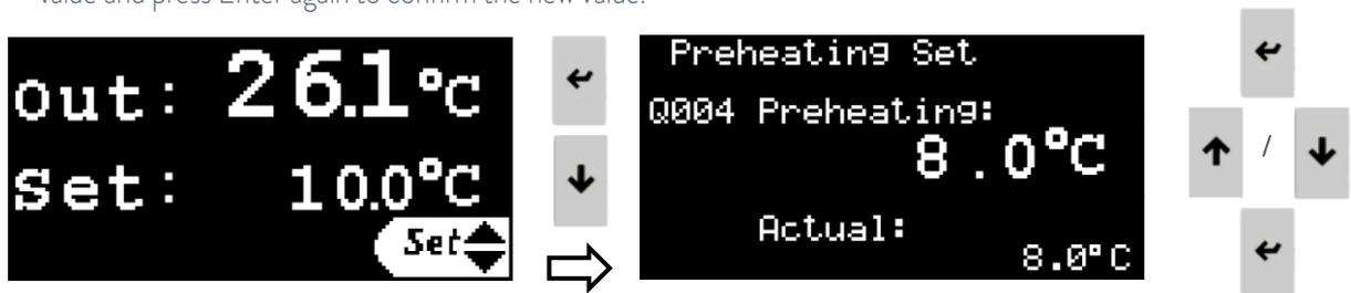
Please note that the heat generated by the pump is limited and, depending on the thermal losses in the whole water circuit, it's possible that the temperature cannot reach the preheating setpoint even with the pump running all the time.
