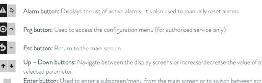
**Enter button:** Used to enter a subscreen/menu from the main screen or to switch between screen navigation and the different parameters that can be modified on a particular screen
