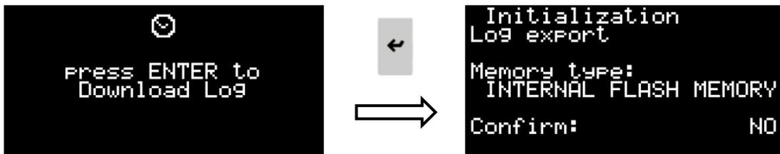
2. Press **Enter** and then the **Up** or **Down** buttons to select where to save the log file. The file can be stored in the chiller's controller Internal Flash Memory or it can be saved to a connected USB drive.
