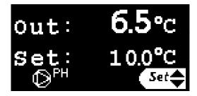
To disable the preheating system, leave it set at the minimum possible value ( $-15^{\circ}$ C,  $5^{\circ}$ F).
