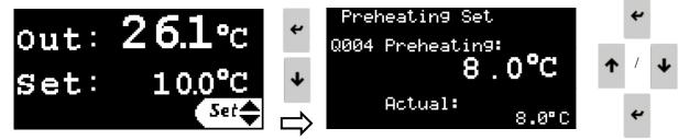
Please note that the heat generated by the pump is limited and, depending on the thermal losses in the whole water circuit, it's possible that the temperature cannot reach the preheating setpoint even with the pump running all the time.
