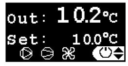
The main screen shows the current outlet temperature, the current setpoint and it shows which motors in the chiller are currently running.
