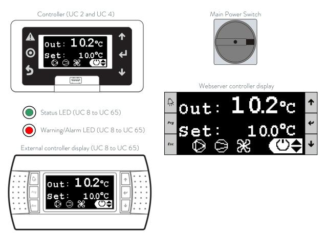
The following elements allow controlling the chiller and monitoring its status:
