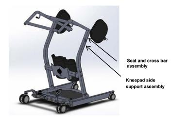
6. Insert the seat and cross bar assembly into the tubes at the top of the kneepad side support assembly as shown above.
