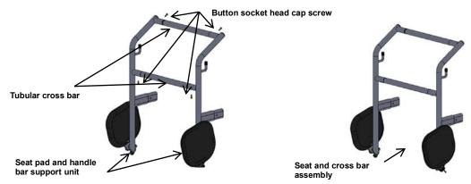
4. Insert the two tubular cross bars into the holes on the seat pad and handle bar support units as shown above. Align the small holes on the cross bar undersides with the holes in the support units. Install the four button socket head cap screws through the support units into the cross bars. Use the hex key to tighten. The finished assembly is shown at right above.
