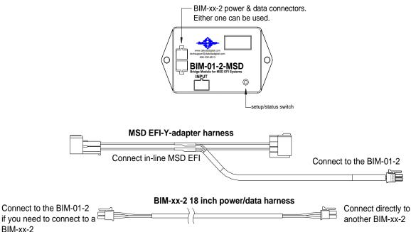
This Bus Interface Module is designed to read engine information from MSD Atomic EFI TBI kits. Atomic EFI LS is <u>not</u> compatible. This module is connected to the MSD EFI through the included Y-adapter harness. This can be plugged in line with the Atomic handheld display or the throttle body.
