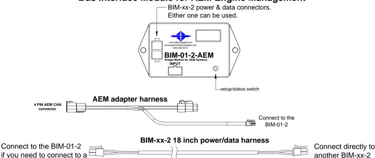
This Bus Interface Module is designed to read engine information from specific AEM CAN bus (AEMnet) enabled devices. These kits include Infinity ECU, Series 2 EMS or EMS-4. The module is connected to the AEM device through the 4-pin
