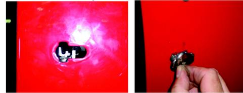
Looking through the lock cylinder hole on the door you will see the slot the pin is to slide into. Make sure the pin is lined up and carefully install the lock cylinder.
