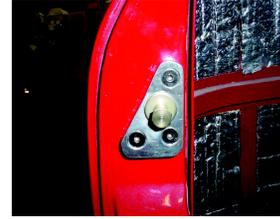
Place the new striker in the door jam and check for alignment.
