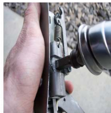
Fig. 2a Test fit shaft to latch
