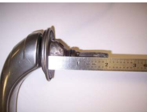
Fig. 1 Measure 2" from base with no gasket. Mark and cut shaft. If you are using a gasket you will need to add the gasket thickness to the length of the shaft.
