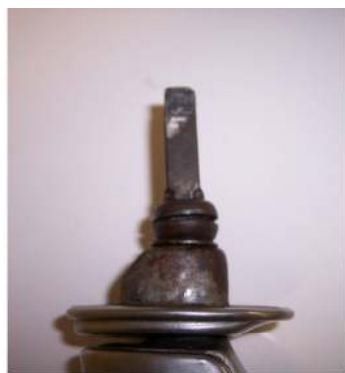
Fig. 2 File or sand shaft to size
