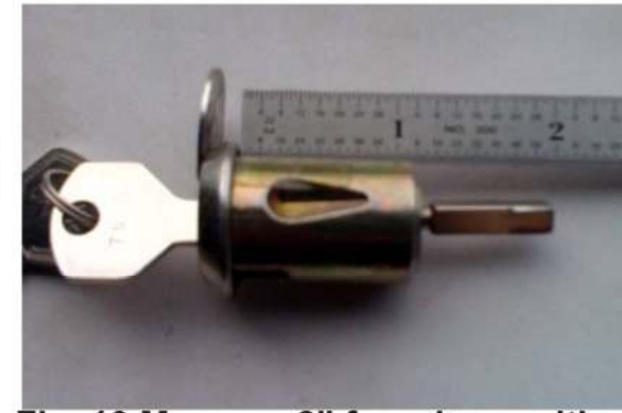
Fig. 10 Measure 2" from base with no gasket. Mark and cut shaft. If you are using a gasket you will need to add the gasket thickness to the length of the shaft.
