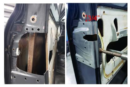
From the center of the window tracks upper mounting hole, measure down 3/4" and make a mark. This will be a reference for the top edge of your installation plate.
