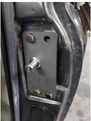
**SLOWLY**, close the door making sure to pay close attention to how the latch aligns to the striker bolt. Using the 4 mounting bolts, adjust the striker plate, so that the striker bolt does not hit any part of the latch or latch plate as the latch clasps closed on it. Make small adjustments to your striker plate until the latch closes easily and your body lines and body panels are properly aligned.
