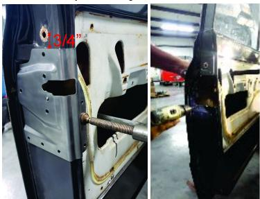
Using the included  $\frac{1}{4}$ -20X3/4 button head bolts and  $\frac{1}{4}$ " hex nuts, attach your installation plate securely to the door.
