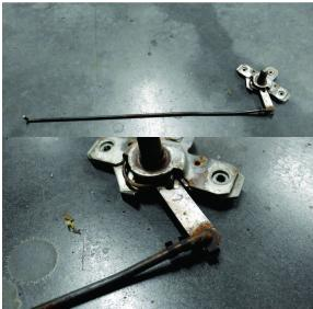
Do not attach the interior door rod to the latch yet. This will be done inside the door.
