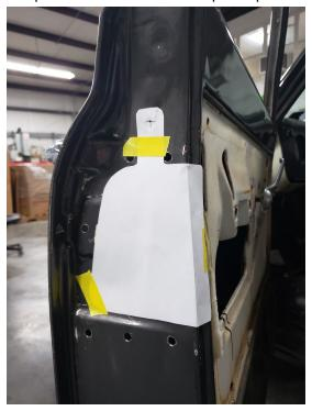
Remove your template and close the gap in your cut line where the template tab was. To make your cut easier, it is advised that you drill a  $\frac{1}{4}$ " hole inside each corner of your cut line. This will give you start and stop points for your saw.
