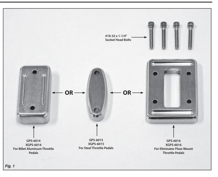
**Step 3:** Position the Throttle Pedal with the Throttle Pedal Spacer on the vehicle, and install the bolts (and nuts if required).
