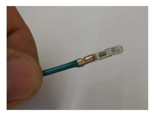
Finally, fold the two rear ears over the insulation and firmly crimp both sets of ears securely to the wire.
