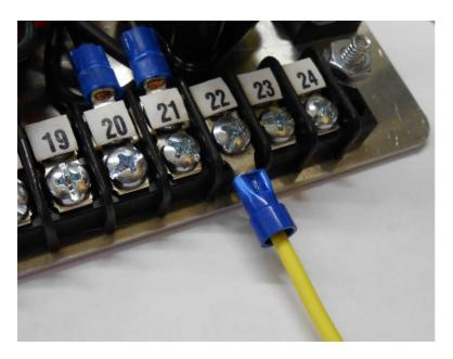
As you continue adding wires to the Power Panel II, you will eventually find that a second wire may need to connect under the same numbered screw. If you installed the first terminal "Face Down" it will be simple to install the next terminal "Face Up." It should not be necessary to install more than two terminals under the same numbered screw on the panel.
