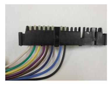
The photo above shows the 4 1/4" male steering column connector properly installed on the steering column wires.
