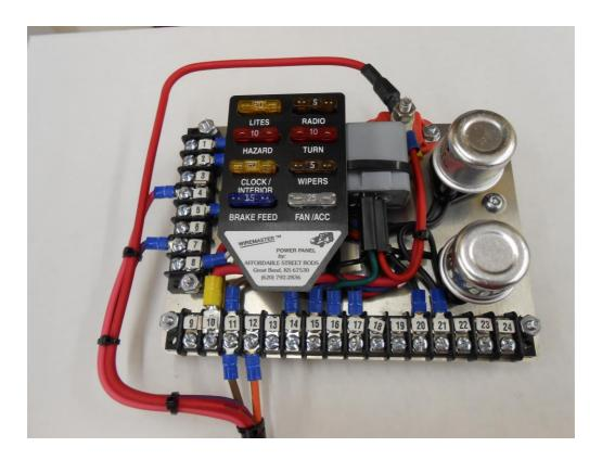
With the Ignition Pigtail connected to the Power Panel II, the pigtail can be cut to length. Be sure to leave enough length to avoid potential chafing against brake pedal, clutch pedal and gas pedal mechanisms.
