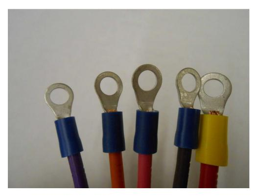
Our universal ignition switches (Part # WRM 30100) have screw terminal connections. The photo above shows ring terminals installed on the five ignition pigtail wires. Other switches may require other types of terminals.
