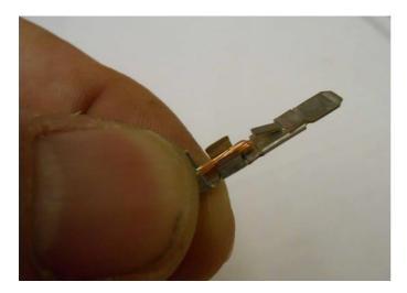
The photo above shows a steering column wire with ½" of insulation stripped and the steering column connector brass terminal held in place.
