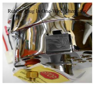
Remove rubber plug from one-wire alternator and snap alternator plug into place.
