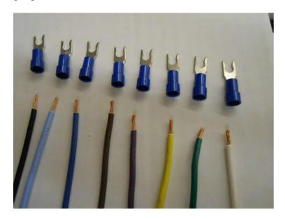
With the steering column pigtail cut to length, strip and crimp one blue fork terminal onto each of the wires and connect the steering column pigtail to the Power Panel II in the following sequence: Black = #17, Light Blue = #18, Blue = #19, Brown = #20, Purple = #21, Yellow = #22, Green = #23, White = #24. We suggest using zip ties to hold the pigtail securely in its final location.
