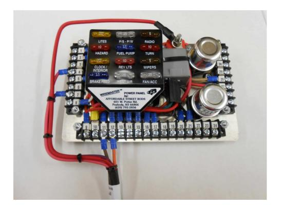
With the Ignition Pigtail connected to the Power Panel, the pigtail can be cut to length. Be sure to leave enough length to avoid potential chafing against brake, clutch and gas pedal mechanisms.
