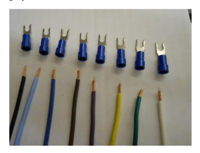
With the steering column pigtail cut to length, strip and crimp one blue fork terminal onto each of the wires and connect the steering column pigtail to the Power Panel in the following sequence: Black = #17, Light Blue = #18, Blue = #19, Brown = #20, Purple = #21, Yellow = #22, Green = #23, White = #24. We suggest using zip ties to hold the pigtail securely in its final location.
