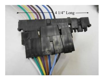
The photo above shows the long flat steering column connector that is present on '77 or later GM columns as well as most after-market columns (except Ididit). The flat connector is 4 ½" long. If your column has this connector, simply plug the Steering Column Pigtail to the column. Make sure that terminal "P" on the female connector aligns with terminal "P" on the male connector and the wire colors should match.
