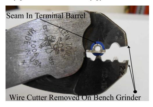
There are a couple of things to note in the previous photo. These pliers come with a wire cutter on the end that we remove with a bench grinder. These pliers produce a superior crimp but we find that it is pretty easy to inadvertently cut one wire while crimping another. Also note how the terminal end is positioned in the pliers. Place the terminal in the jaws so that the seam in the terminal barrel is in the concave jaw. This method of crimping insures a tight trouble-free crimp.
