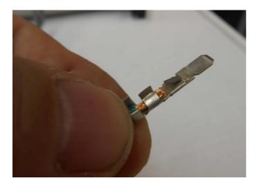
Start crimping the steering column connector brass terminal onto the wire by folding one forward ear over the stripped wire.
