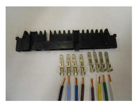
The photo above shows the eight wires from the steering column stripped and ready for installation of the steering column connector brass. With brass terminals crimped to each of the wires, insert them into the connector as follows: White = P, Green = N,
