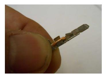
The photo above shows a steering column wire with ½" of insulation stripped and the steering column connector brass terminal held in place.
