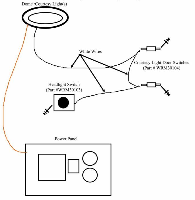
Courtesy lights are wired to be hot all of the time. The courtesy light door switches (Part#WRM30104) create a ground for the light(s) when the door(s) are opened.
