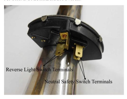
Pictured above is a Flaming River column-shift column with a combo neutral safety switch and reverse light switch. Stock GM column-shift columns will use a similar switch.
