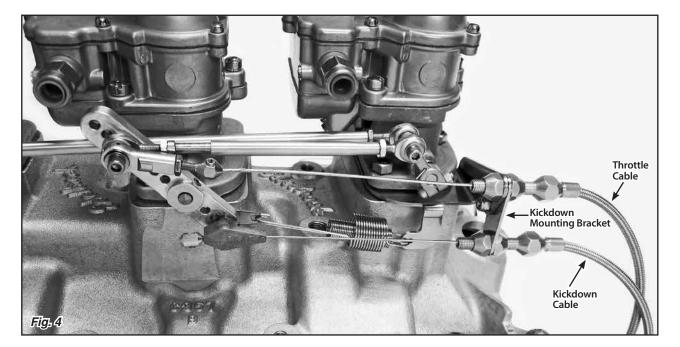
Throttle Cable and Kickdown Cable not included. Both are available separately. The Kickdown Mounting Bracket is part of the Kickdown Kit.
