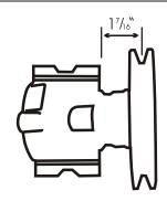
1-7/16" center of pulley groove to front side of mounting hole
