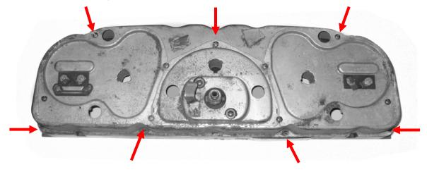
2. Remove the stock gauges, separator plate, and lens from the bezel. The only item to be reused is the original front bezel; the other pieces can be set aside. Cut the supplied foam tape into four pieces, so each is about two inches long. Cut them lengthwise to make eight thin strips; stick the foam strips on the angled part of the inside edge of the bezel. The lens will compress against any foam above the edge, which helps prevent lens rattles.
