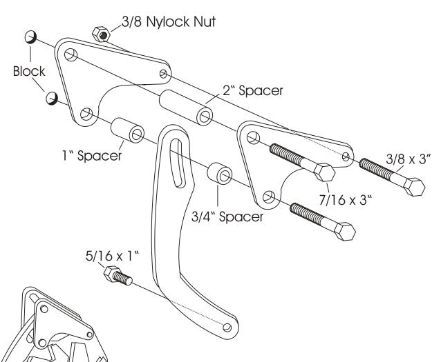
(We use a belt length of 43-44" with this mount on installations in our shop. However; this can vary with the diameter of your pulleys.)
