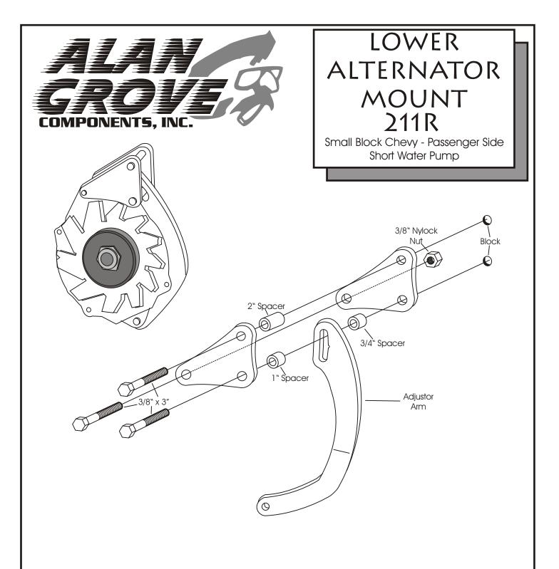
(We use a belt length of 42 to 43" with this mount on installations in our shop. However; this can vary with the diameter of your pulleys.)
