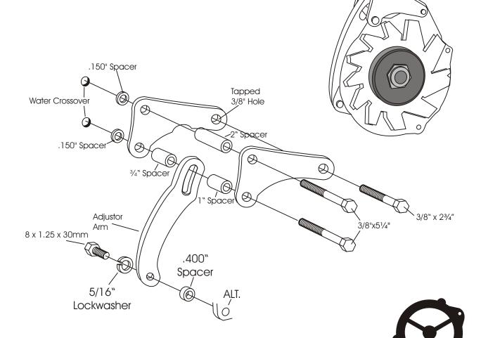
(We use a belt length of  $41\frac{1}{4}$  to 42° with this mount on installations in our shop. However; this can vary with the diameter of your pulleys.)
